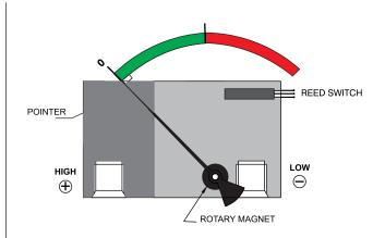
Instrument consists of a convoluted diaphragm to sense the pressure difference. It can withstand maximum operating pressure up to 100 bar for all ranges. If pressure exceeds the rated maximum pressure, "O" rings & diaphragm inside the pressure chamber, will be damaged. If maximum operating pressure is within the allowable limit of 100 bar, but the differential pressure exceeds instrument range, there will be no damage to the instrument. Pointer will only go the extreme right end of the scale.
